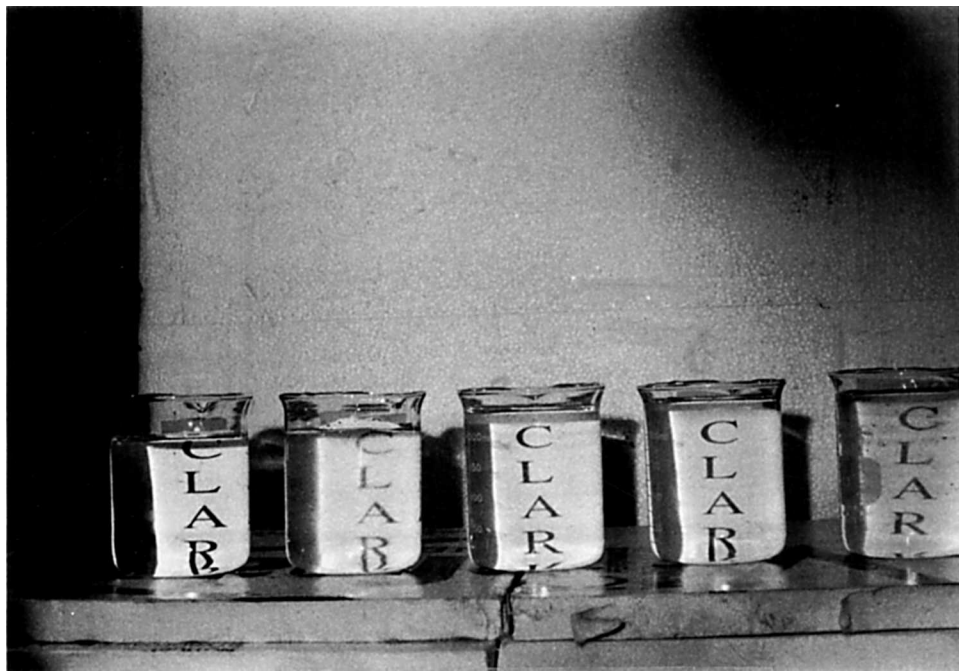
Figure 6 Clarity comparison of distilled water with D-10-G400 HSPAN gel-distilled water dispersion. Left to right: distilled water, new dispersion, dispersion heated at 60°C, dispersion heated at 73°C, and dispersion heated at 70-78°C.
